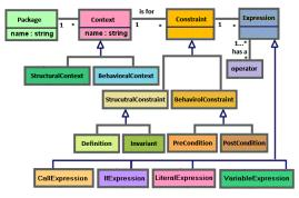
Figure 1. Elements of selected OCL meta-model
