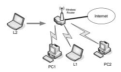
Figure 3: Wireless Router used in a PAN
