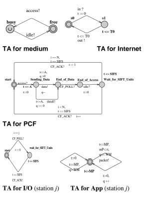
Figure 6: Behavioural Model of the system
