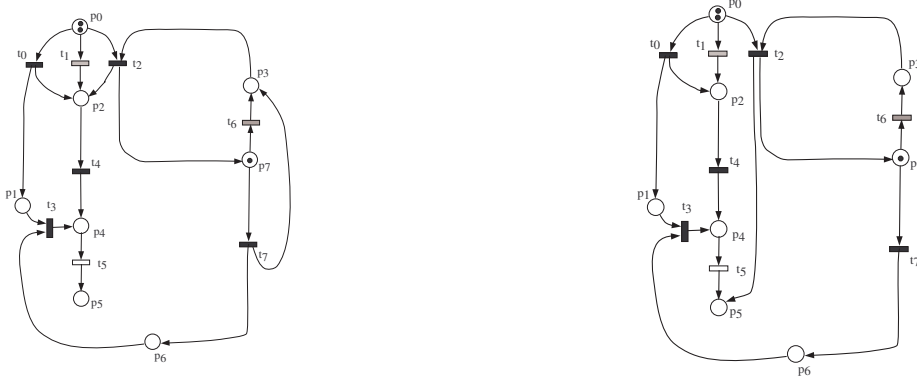
Fig. 6. A a PN with trap unobservable circuits (left) and a general PN (right)
